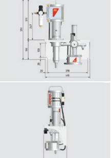
The compressed air driven piston pump delivers with upwards and downwards strokes and thereby creates an extremely consistent glue pressure. Due to quick regulation, the glue application remains constant even during changes in the production speed. The integrated pressure monitor automatically initiates an alarm if the pressure deviates from the set value. A fine filter at the pump output traps the smallest foreign particles and protects the dispensing system.
